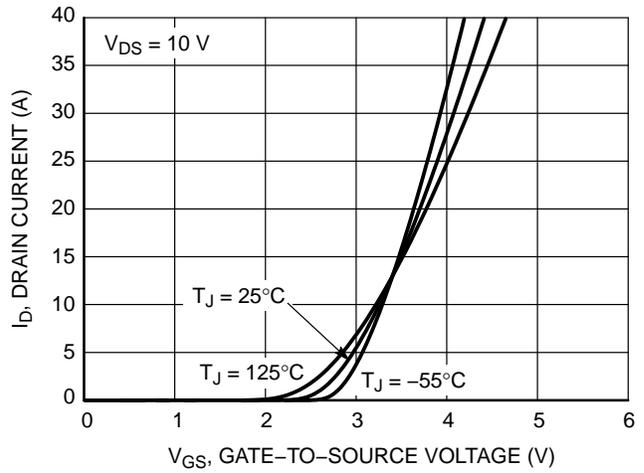
Figure 2. Transfer Characteristics
