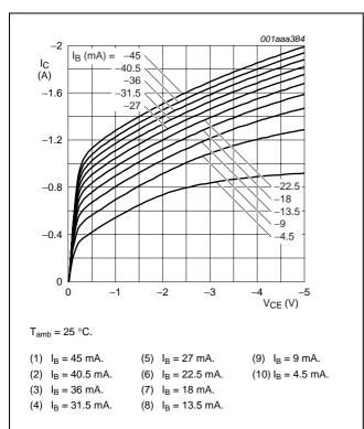
Fig.13 Collector current as a function of collector-emitter voltage; typical values.
