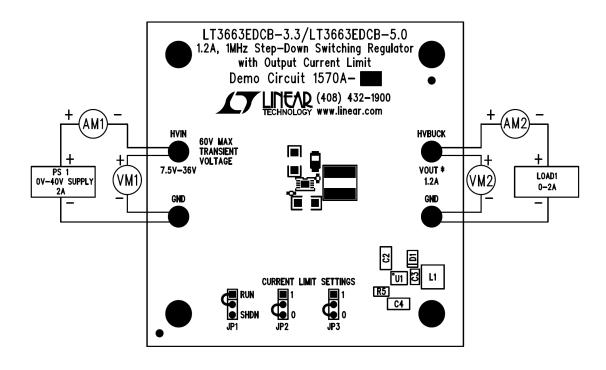
**Figure 1: Proper Measurement Equipment Setup**
