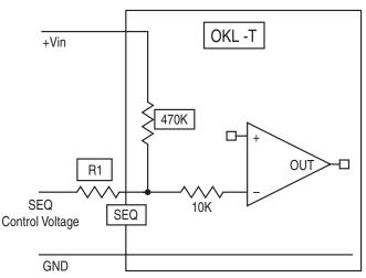
Figure 6. Sequencing Signal Interface of Module
