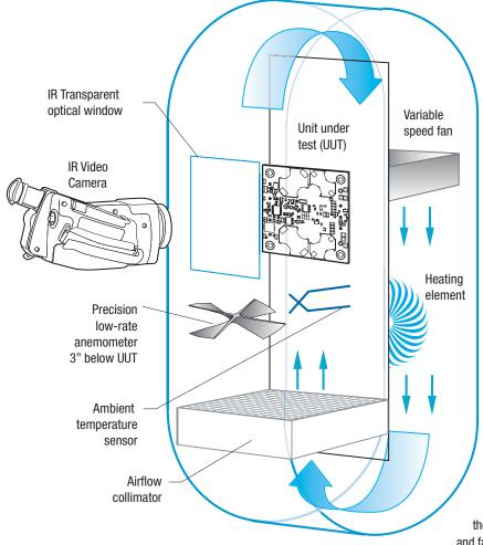
Figure 9. Vertical Wind Tunnel
