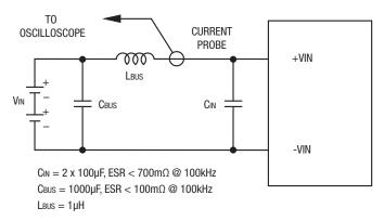
Figure 4: Measuring Input Ripple Current
