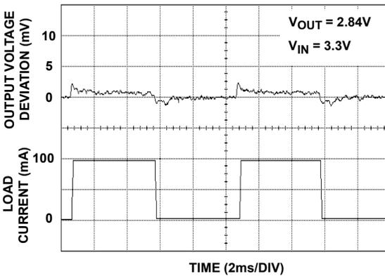
FIGURE 7. LOAD TRANSIENT RESPONSE ( $V_{OUT2}$ )
