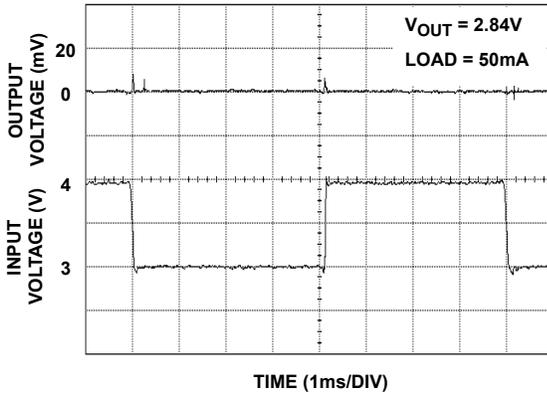
FIGURE 5. LINE TRANSIENT RESPONSE ( $V_{OUT3}$ )
