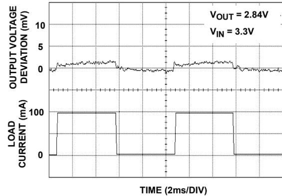
FIGURE 8. LOAD TRANSIENT RESPONSE ( $V_{OUT3}$ )
