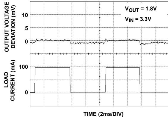
FIGURE 6. LOAD TRANSIENT RESPONSE ( $V_{OUT1}$ )
