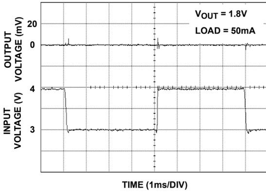
FIGURE 3. LINE TRANSIENT RESPONSE ( $V_{OUT1}$ )
