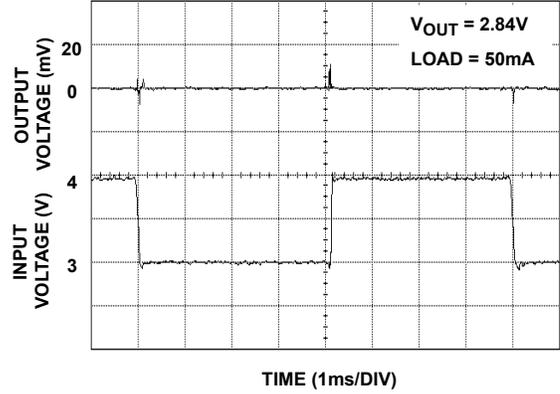
FIGURE 4. LINE TRANSIENT RESPONSE ( $V_{OUT2}$ )
