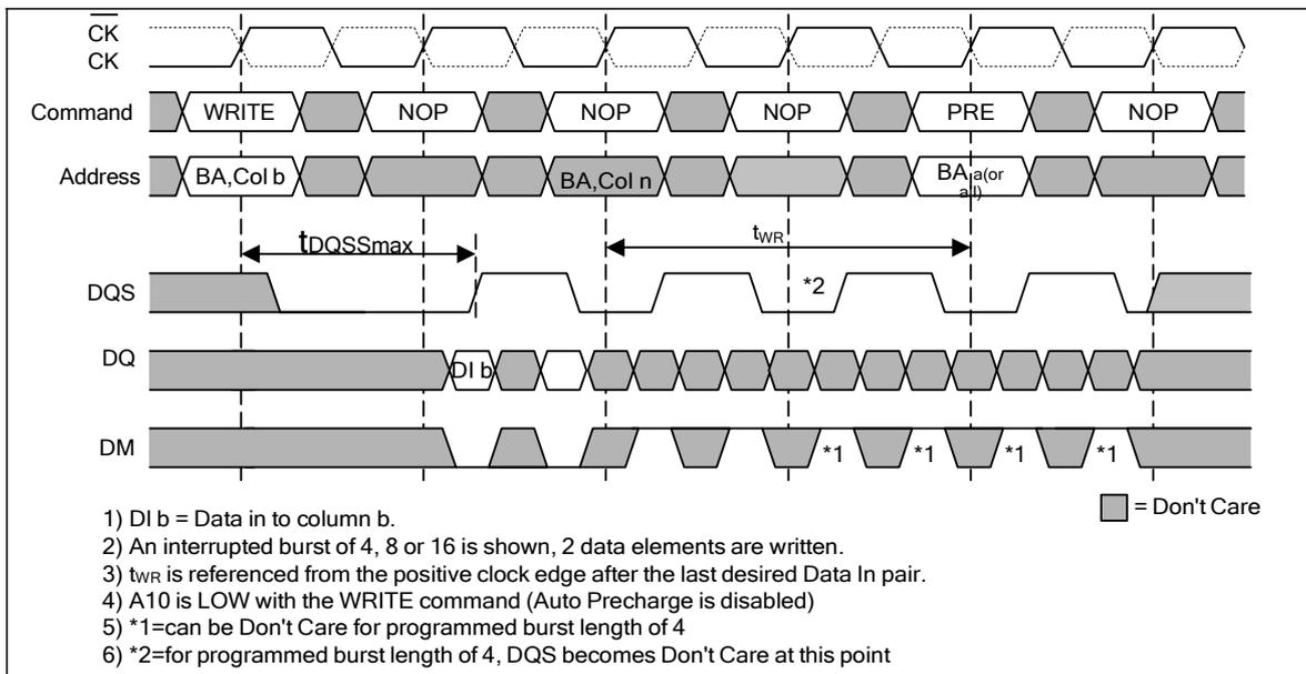
**Figure 31 — Interrupting Write to Precharge**
