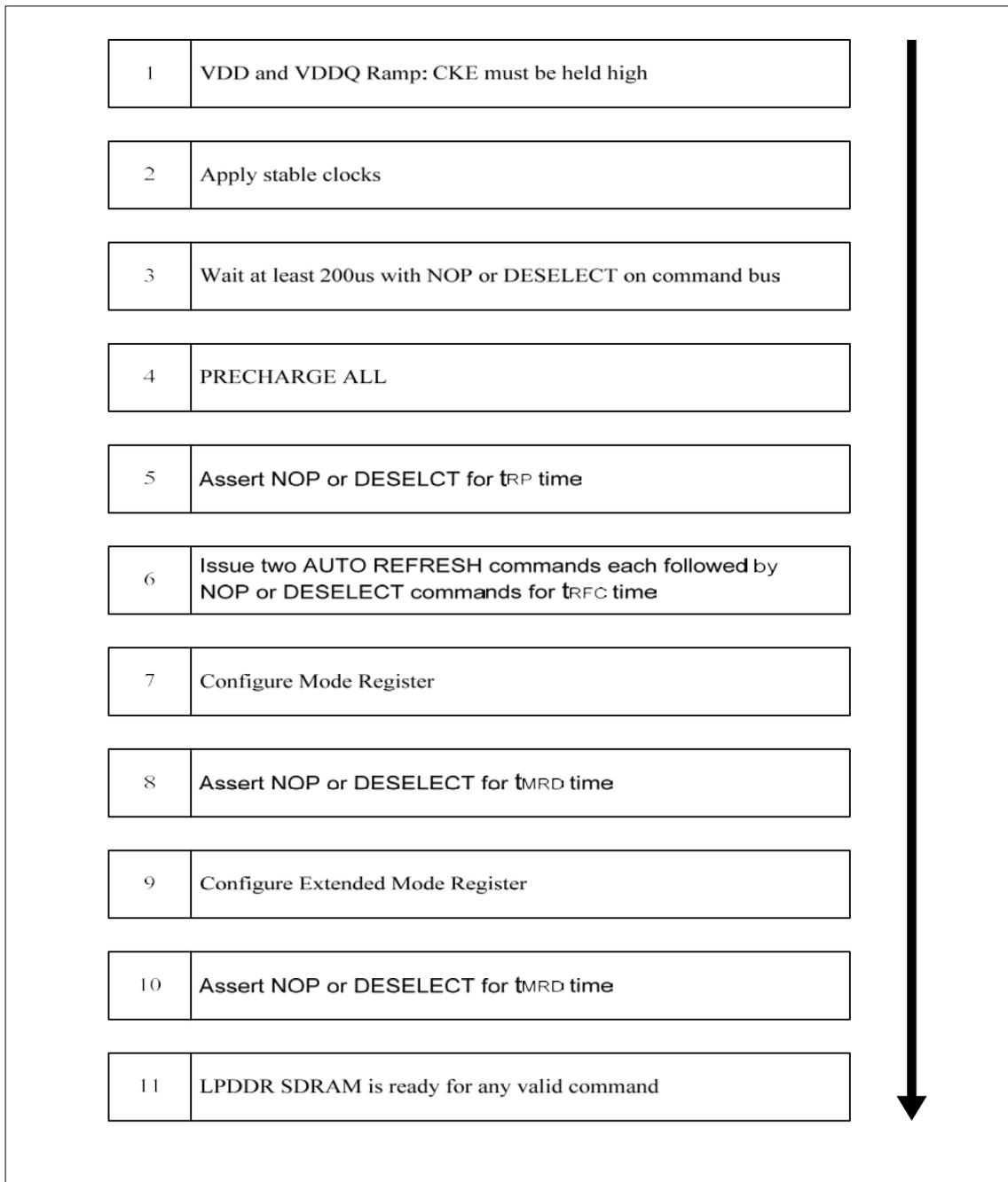
**Figure.4 — Flow Diagram**
