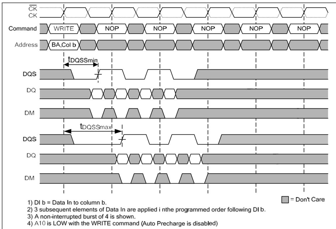
**Figure 24 — Write Burst (min. and max. tDQSS)**
