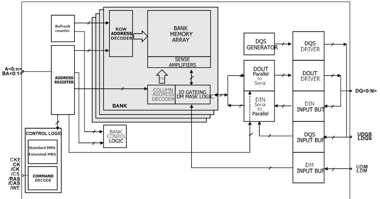
Figure.2 — Block Diagram
