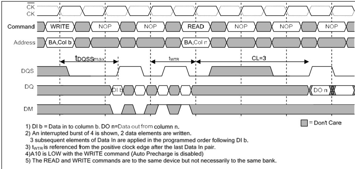
**Figure 29 — Interrupting Write to Read**
