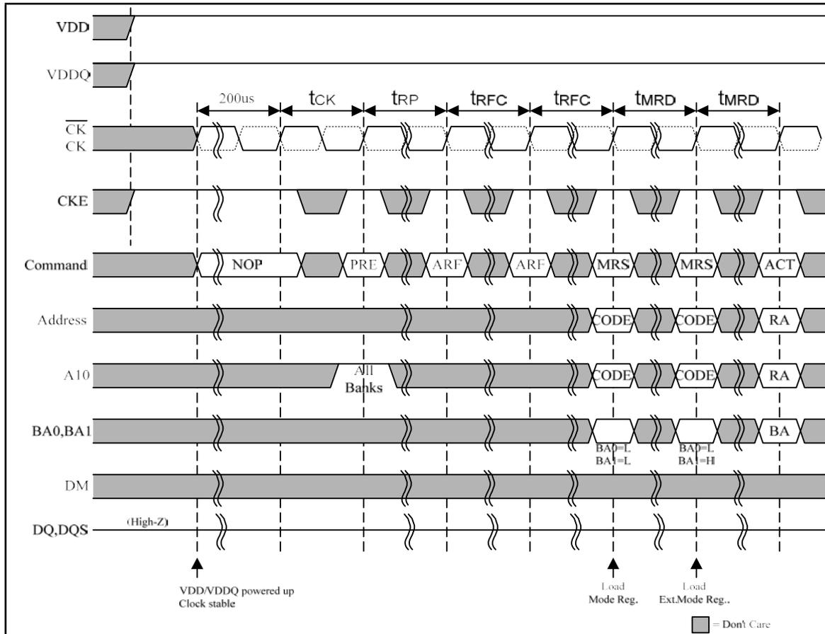
**Figure 5 — Initialization Waveform Sequence**
