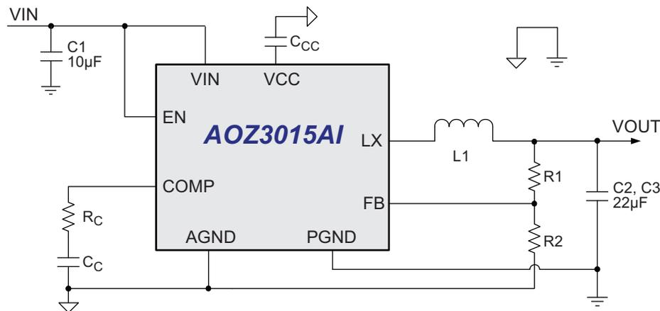
Figure 1. 3 A Synchronous Buck Regulator,  $F_s = 500 \text{ kHz}$
