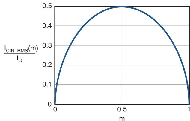
Figure 2. I<sub>CIN</sub> vs. Voltage Conversion Ratio
