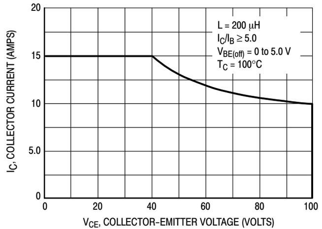
Figure 3. Maximum Rated Forward Bias Safe Operating Area
