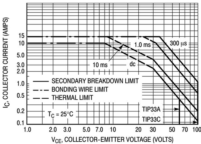
Figure 2. Maximum Rated Forward Bias Safe Operating Area
