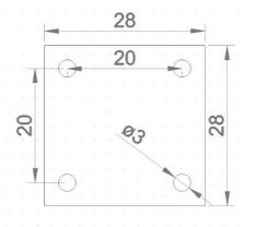
All dimensions in mm. Tolerance 0.1mm. All mounting holes are on 10mm spacings.
