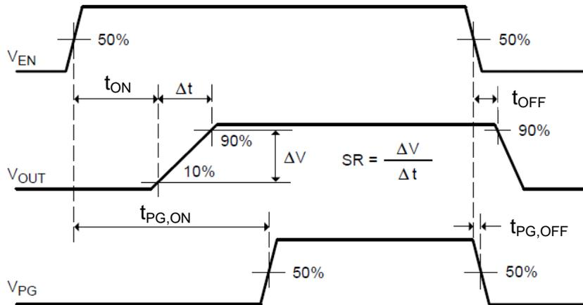
Figure 1 Timing Diagram
