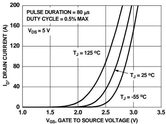
**Figure 5. Transfer Characteristics**
