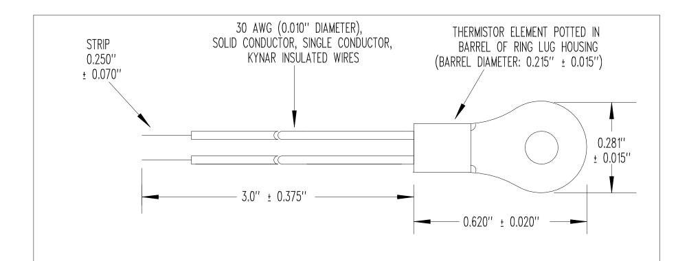
RESISTANCE @  $+25^{\circ}\text{C} = 10,000 \ \Omega \pm 5\%$ RESISTANCE/TEMPERATURE CURVE = ''J'' TEMPERATURE COEFFICIENT @  $+25^{\circ}\text{C} = -4.4\%$ /'C NOMINAL BETA '' $\beta$ '' (0 TO  $+50^{\circ}\text{C}$ ) = 3,892'K NOMINAL MAXIMUM TEMPERATURE RATING =  $+125^{\circ}\text{C}$
