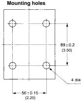
Note: Mounting hole diameter varies with the panel thickness and material. The table below is for soft iron panel.
