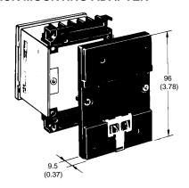
The H5S-FB timer can be mounted on DIN rail track using the Y92F-90 adapter. Two screws supplied with the timer fasten the adapter to the timer.
