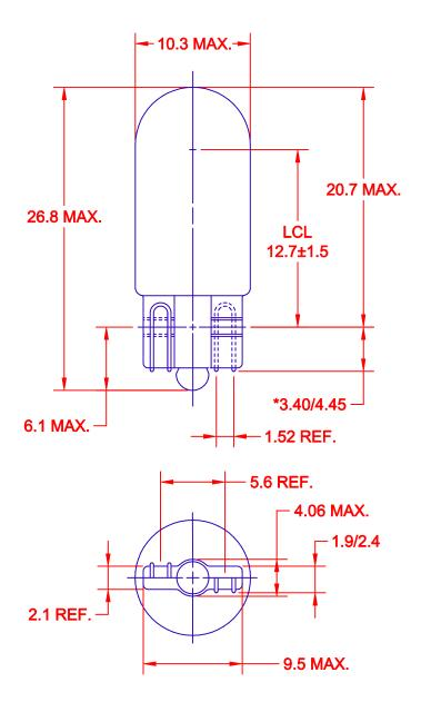
\*TO BE MEASURED ON LONGEST SIDE ONLY WITH THE WIRE IN INTIMATE CONTACT WITH THE BOTTOM OF THE GLASS WEDGE.
