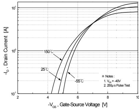
**Figure 2. Transfer Characteristics**
