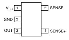
The very low offset voltage enables a typical accuracy of 1% for sense voltages of only 30mV, giving better tolerances for small sense resistors necessary at higher currents.
