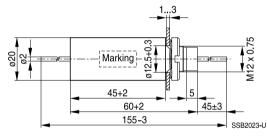
Tightening torque: 4 +0.5 Nm
