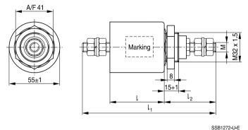
General tolerances according to ISO 2768-cL Dimensions in mm
