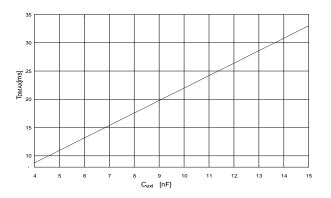
Figure 6:  $T_{\text{DMAX}}$  as function of external CSSD capacitor
