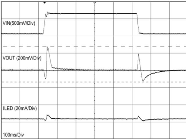
Figure 10. Line Transient Response for 6 LEDs
