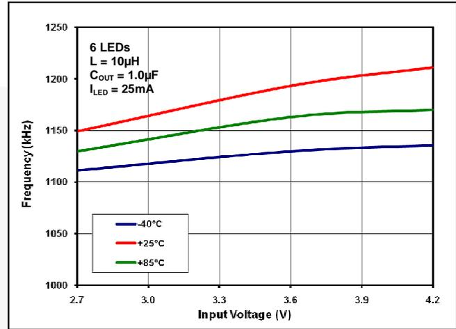
Figure 5. Frequency vs. Input Voltage vs. Temperature
