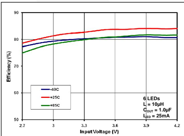
Figure 8. Efficiency vs. Input Voltage vs. Temperature
