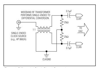
Figure 4. Differential Clock Signal Generation
