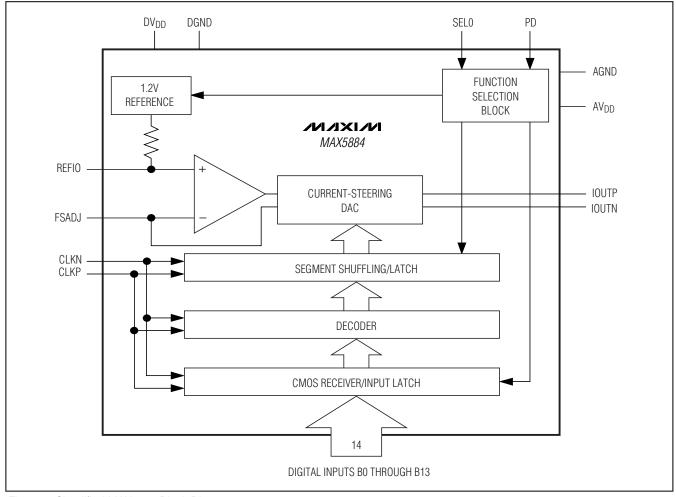
Figure 1. Simplified MAX5884 Block Diagram
