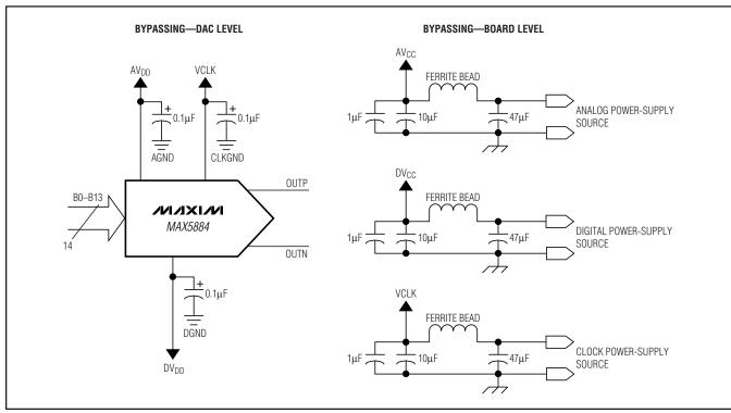
Figure 12. Recommended Power-Supply Decoupling and Bypassing Circuitry
