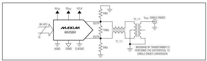
Figure 6. Differential to Single-Ended Conversion Using a Wideband RF Transformer
