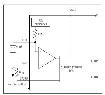
Figure 2. Reference Architecture, Internal Reference Configuration
