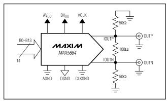
Figure 7. MAX5884 Differential Output Configuration
