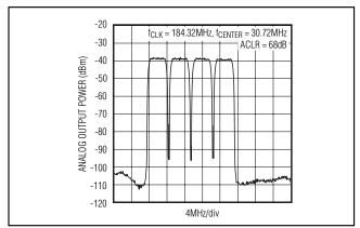
Figure 9. ACLR for W-CDMA Modulation, Four Carriers
