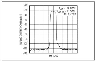
Figure 8. ACLR for W-CDMA Modulation, Single Carrier
