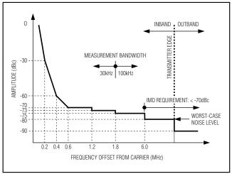
Figure 10. GSM/EDGE Tx Mask Requirements
