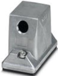
HEAVYCON ADVANCE sleeve housing, B10, with stainless steel screw locking (Allen screw), salt-water-resistant aluminum, height 74 mm, with 1x M20 thread, lateral cable outlet, without surface, conductive seal (EMC properties)
