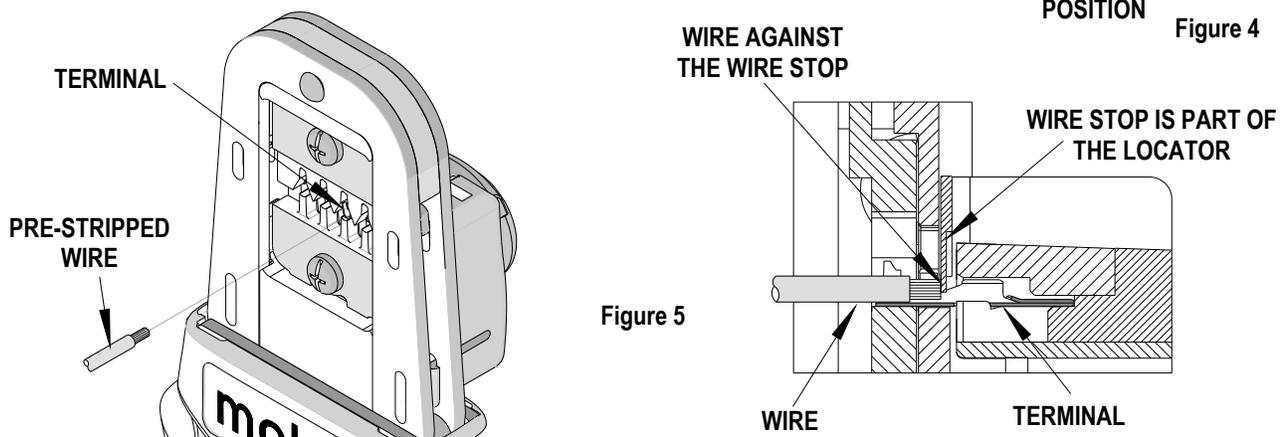
**Note: The tamper proof ratchet action will not release the tool until it has been fully closed.**
