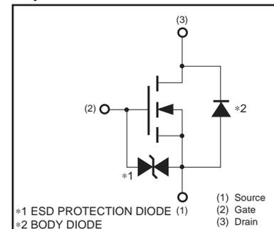
\* A protection diode has been built in between the gate and the source to protect against static electricity when the product is in use. Use the protection circuit when fixed voltages are exceeded.
