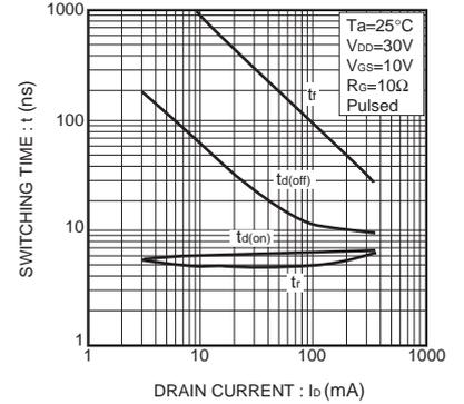
Fig.12 Switching Characteristics
