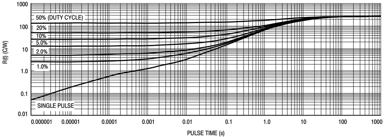
Figure 8. Thermal Response, Junction-to-Ambient (6 mm<sup>2</sup> pad)
