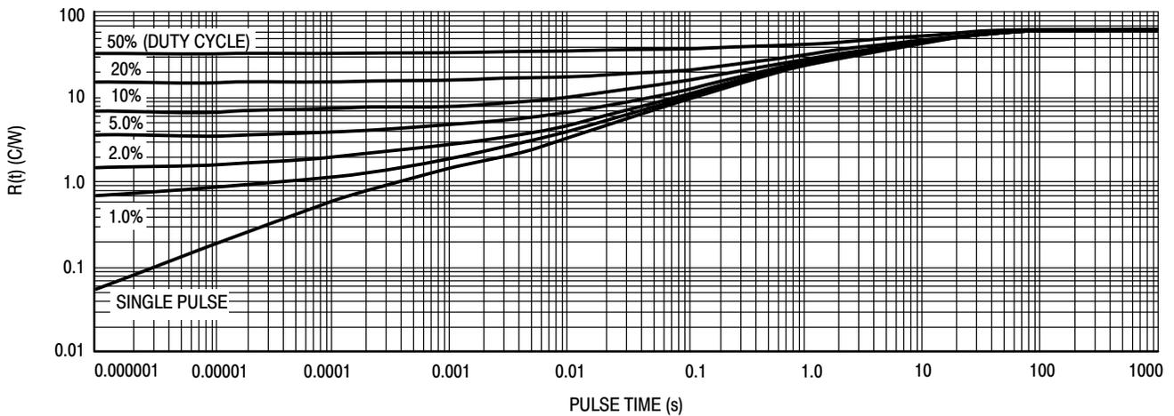
Figure 9. Thermal Response, Junction-to-Ambient (1 in<sup>2</sup> pad)
