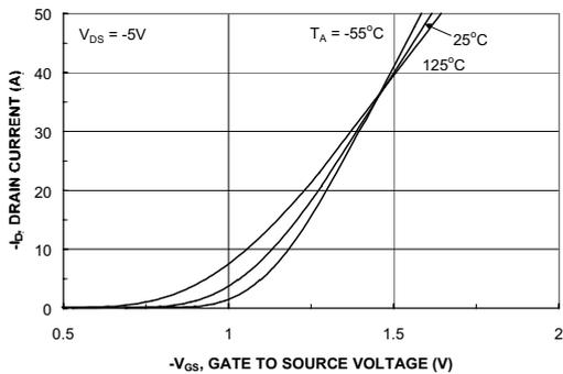
Figure 5. Transfer Characteristics.
