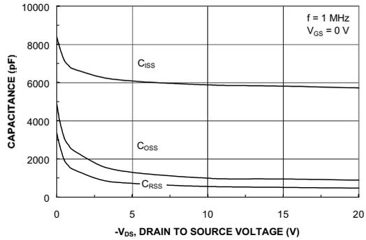
Figure 8. Capacitance Characteristics.
