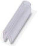
Conductor marker carrier, transparent, unlabeled, Mounting type: slide on, Cable diameter: 4-7 mm, Lettering field: 4 x 15 mm
