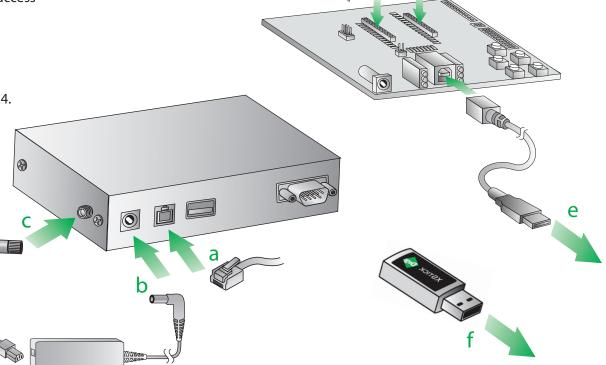
NOTE: If the XStick or XBIB devices are not recognized automatically, you can download the corresponding drivers from the Documentation tab at www.digi.com/tanksolutionskit.
