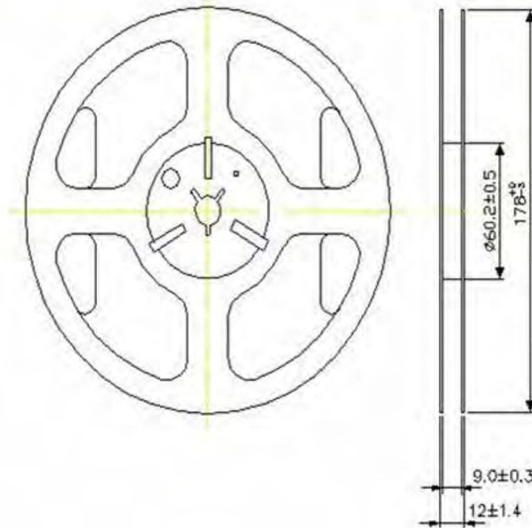
1. 230mm minimum leader which consist of carrier and/or tape followed by a minimum of 160mm of empty carrier tape sealed with cover tape.
