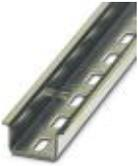
DIN rail, material: steel galvanized and passivated with a thick layer, perforated, height 15 mm, width 35 mm, length: 2000 mm
