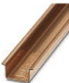
DIN rail, material: Copper, unperforated, 1.5 mm thick, height 15 mm, width 35 mm, length: 2 m
