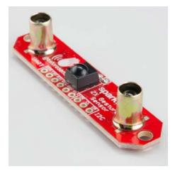
They are held on with Super Glue. You can remove them, but it might require a bit of acetone. If you plan to mount the ZX Sensors in your own housing, make sure IR light can't travel directly from the sides of the LEDs to the receiver (i.e. you will want to make your own IR shields).
