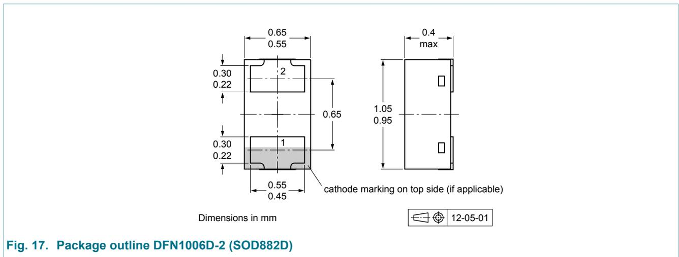
Fig. 17. Package outline DFN1006D-2 (SOD882D)
