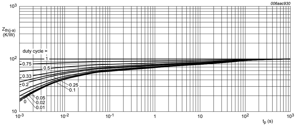
Ceramic PCB, Al<sub>2</sub>O<sub>3</sub>, standard footprint
