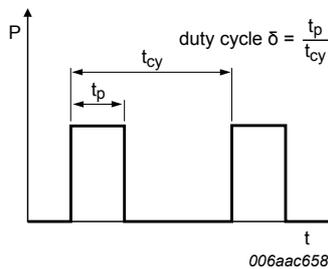
Fig. 16. Duty cycle definition
