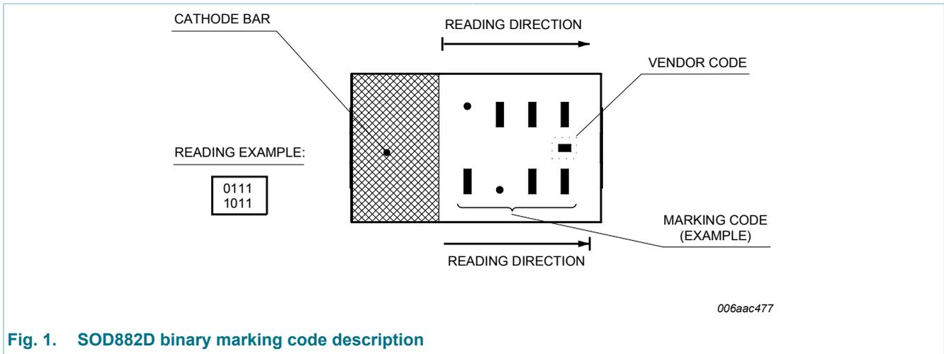
Fig. 1. SOD882D binary marking code description
