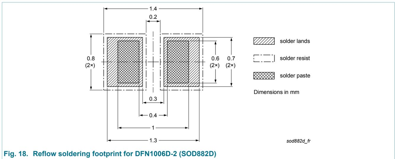
Fig. 18. Reflow soldering footprint for DFN1006D-2 (SOD882D)
