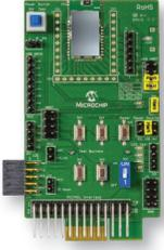
This board enables development with the RN4870 BLE module. The board includes a sensor daughter board for experimentation with on-board light and temperature sensing, a potentiometer, a pushbutton switch and LEDs. The board can be interfaced via USB and any PC terminal program, or over the PICTail interface connected to one of Microchip's microcontroller development boards such as the Explorer 16 Development Board.
