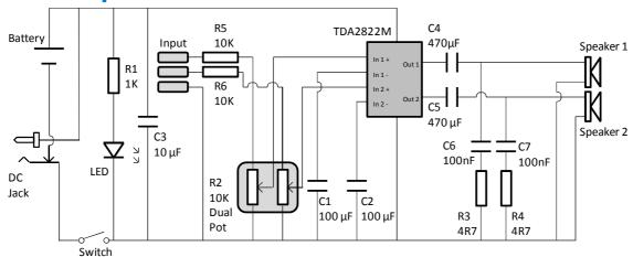
At the centre of the circuit is an audio amplifier Integrated Circuit or IC. Inside the IC are lots of transistors, which are connected together to allow the small input signal to be amplified into a more powerful output that can drive a speaker.
