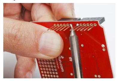
Once all four headers are nice and square, set the board down again and solder the other pins. It pays to start soldering pins as far from the singles that you tacked down earlier as possible; that way, you won't accidentally melt the first one and cause the header to go all wobbly again before it's secured.
