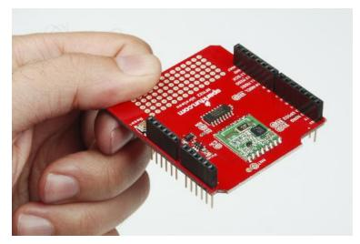
Flip the board over so the male pin side is up. This is the tricky part- the headers have a tendency to rock left to right, so that the end up soldered at a non-right angle with the board, which makes connecting other boards difficult or impossible. Tack down <u>one and only one</u> pin on each header.
