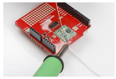
Once the wire is soldered in place, measure 8.3cm (3 1/4 inches) of wire from the underside of the board and snip off the excess. This tunes the antenna to 1/4 of the wavelength of the transmit/receive frequency (910MHz), which gives the best performance/size tradeoff.
