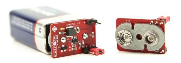
snapVCC is a highly portable and convenient power supply for your electronics projects. It's designed to fit right on a 9V battery and give you 3.3V or 5V power wherever you need it.
