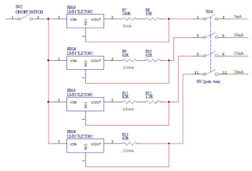
Figure 3.6: LED Constant Current Block Diagram
