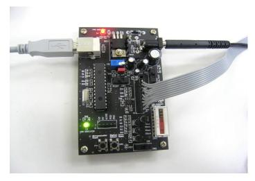
Figure 4.1: Controller board with all interface connected
