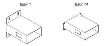
Four Base Mount Kits used in conjunction with the Cub Counter Series are available to replace almost all existing miniature and general purpose electromechanical counters on the market today. Two Base Mount Kits are designed for the CUB1 (BMK1 and BMK1A), one for the CUB2 (BMK2), and one for the CUB3 (BMK5). The kits are coated with a durable flat black polyurethane finish.
