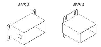
The connecting wires can either be brought through the panel on which the unit is mounted, or through a hole in the enclosure itself. A grommet is provided to insert in the hole on the base mount (where applicable) when wires are routed through it. A plug is provided to close the hole when this option is not used. The plug and grommet are provided in the accessory bag with each base mount unit along with four nuts and bolts for mounting.
