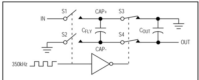
Figure 3. Transferring Charge on C<sub>FLY</sub> to C<sub>OUT</sub>
