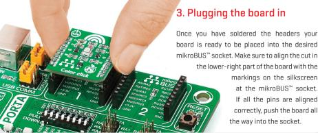
Once you have soldered the headers your board is ready to be placed into the desired
