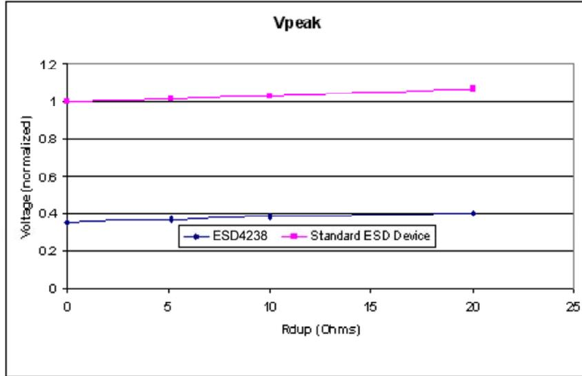
Figure 5. Normalized V<sub>Peak</sub> (8 kV IEC-61000 4-2 ESD Contact Strike) vs. Loading (RDUP)\*
