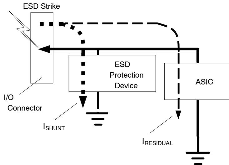
**Figure 2. Standard ESD Protection Device Block Diagram**
