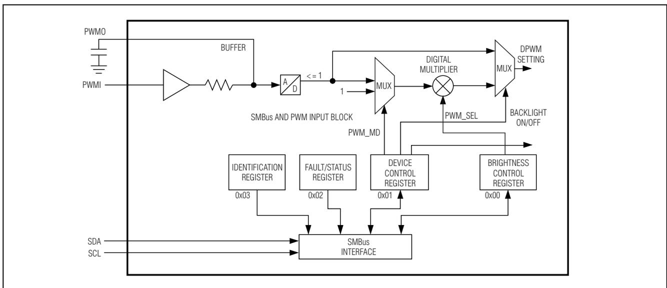
Figure 4. MAX17061A PWM and SMBus Interface Circuit
