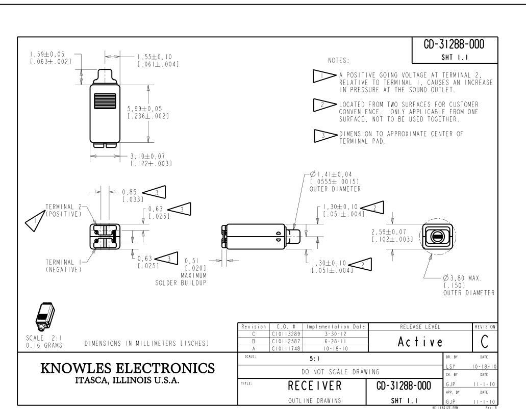
INTENDED FOR USE IN CIC, RIC, AND MINI-BTE APPLICATIONS. THIS IS A PAIR OF GE RECEIVERS WITH VERY LOW VIBRATION IN ALL DIRECTIONS. ONE GE RECEIVER IS REVERSE MAGNETIZED FOR MAGNETIC LEAKAGE CONSIDERATIONS.
