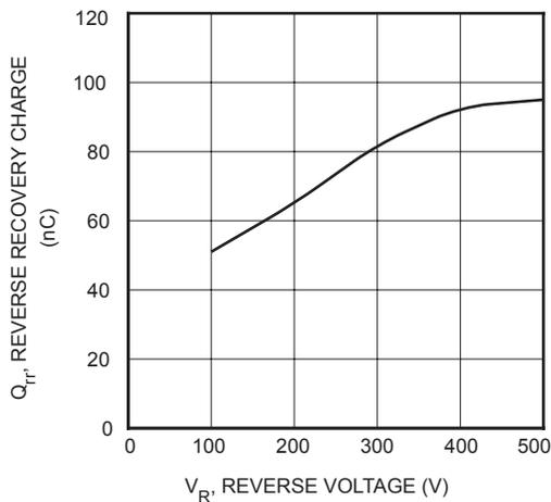
Figure 6. Reverse Recovery Charge vs. V<sub>R</sub>
