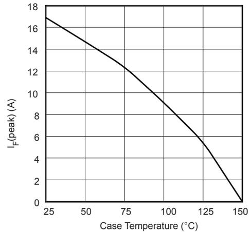
FIGURE 3, Maximum Forward Current vs. Case Temperature
