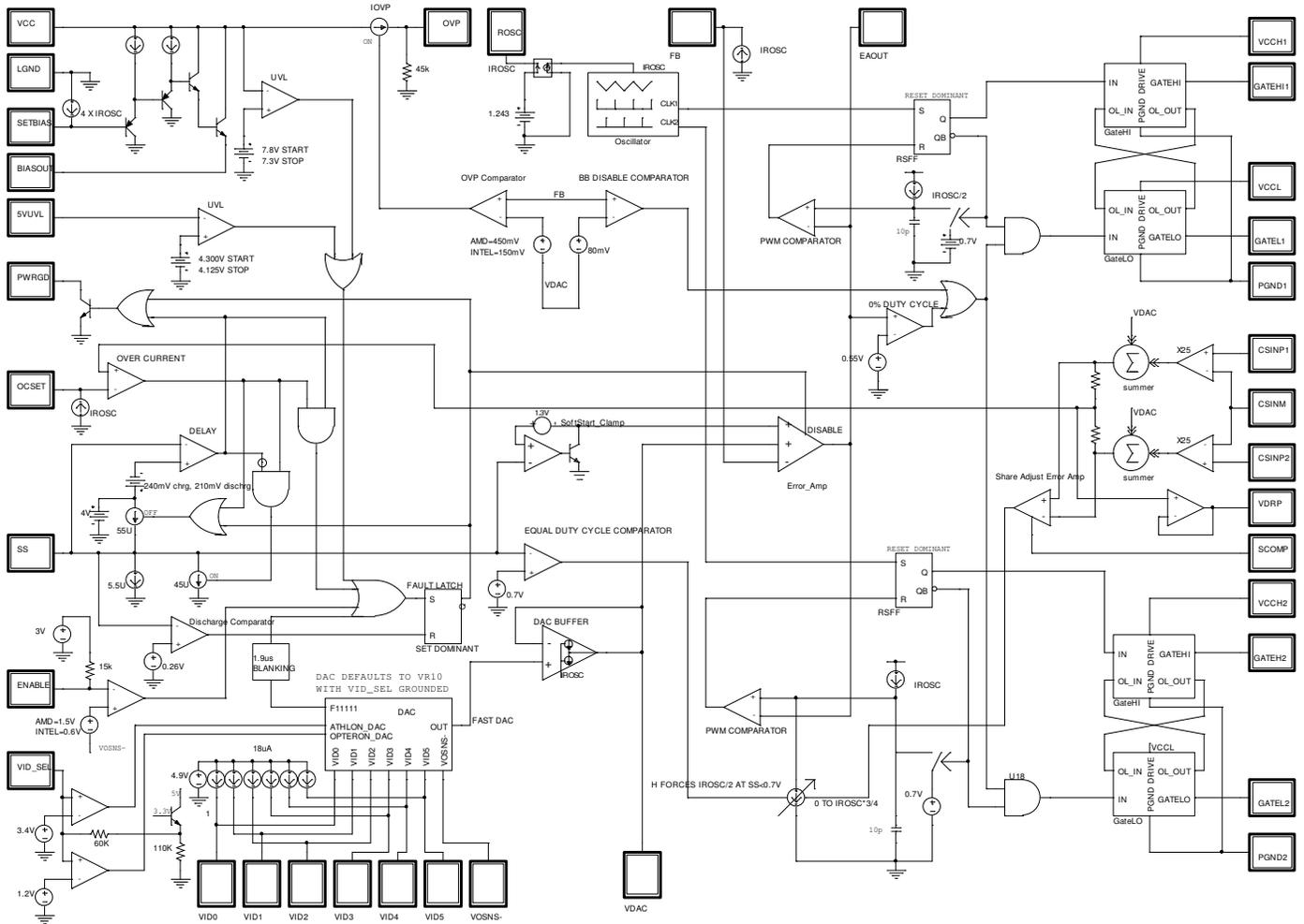
**Figure 1 – IR3092 Block Diagram**
