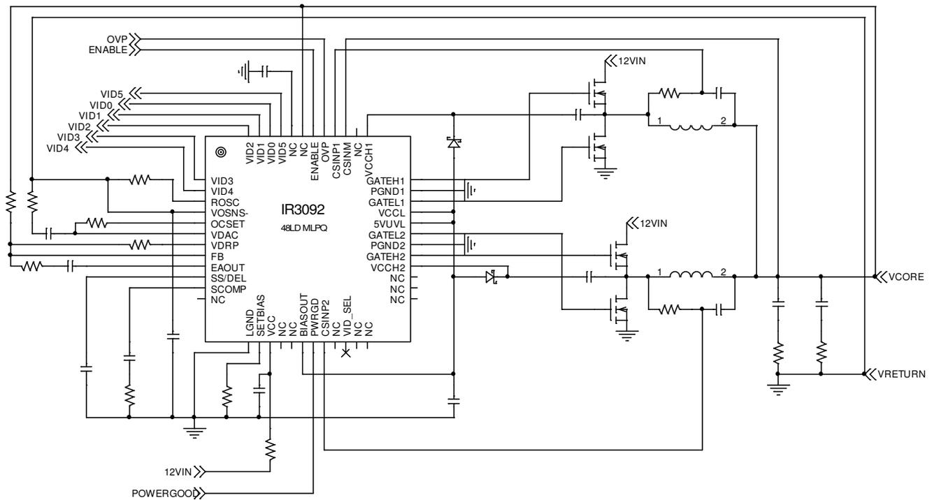
**Figure 12. 12V Control, 12V Power Oteron Converter**
