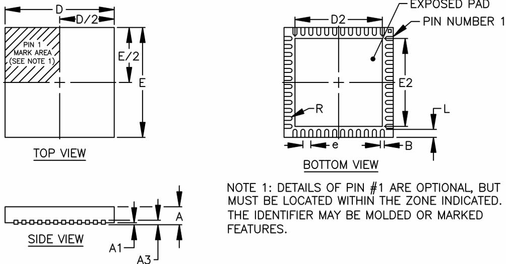
NOTE 1: DETAILS OF PIN #1 ARE OPTIONAL, BUT MUST BE LOCATED WITHIN THE ZONE INDICATED. THE IDENTIFIER MAY BE MOLDED OR MARKED FEATURES.
