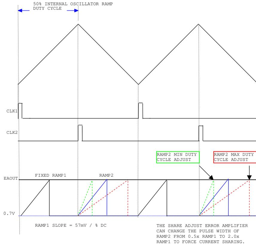
**Figure 3 – 2 Phase Oscillator and PWM Waveforms**
