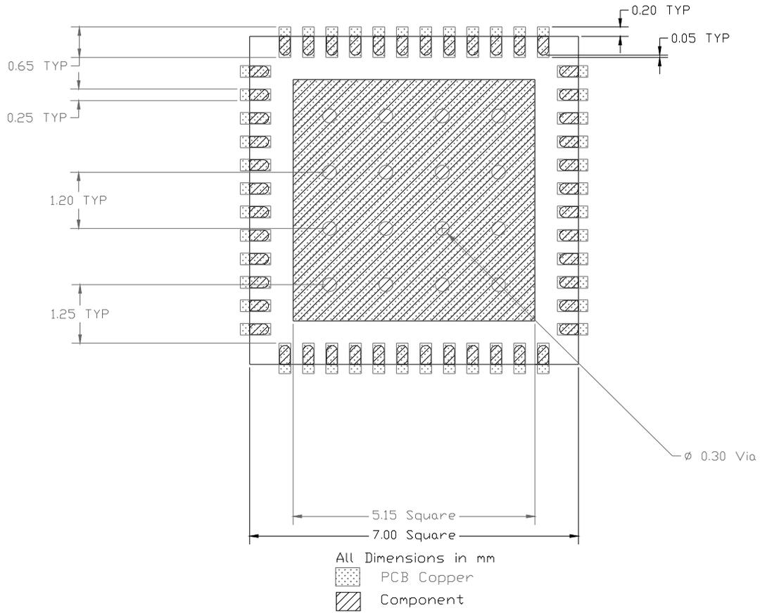
**Figure 15. PCB metal and component placement.**
