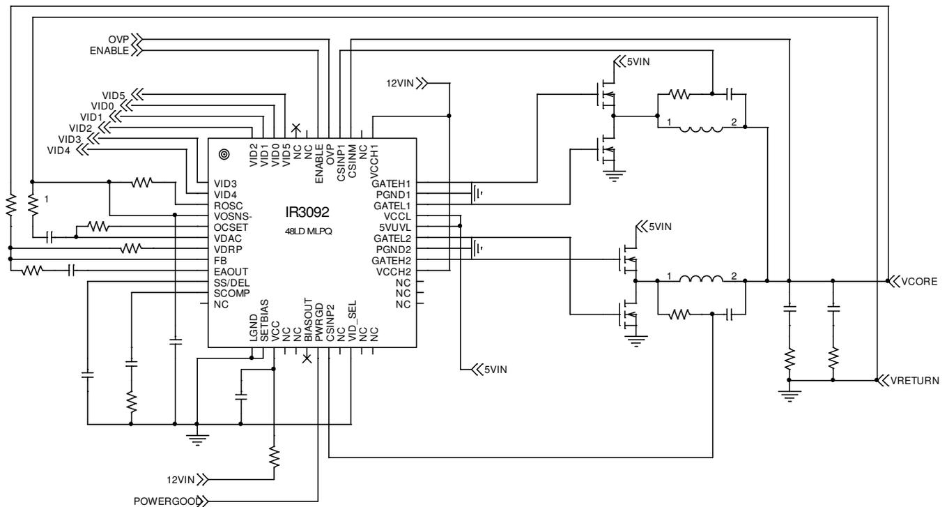
**Figure 13. 12V Control, 5V Power, VR10.0 Converter**
