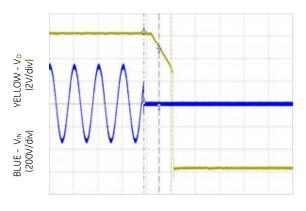
Figure 7. Ride Through at full load,  $V_{IN} = 230V_{ac}$ ,  $V_o = 12V_{dc}$ ,
