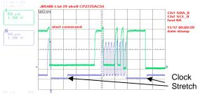
Figure 15. Example waveforms showing clock stretching.
