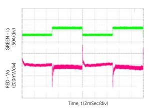
Figure 10. 50%-100%-50% Load Transient, Slew Rate = 1A/uS,  $V_{\rm IN}$  = 230V\_{ac,}  $V_o$  = 12Vdc
