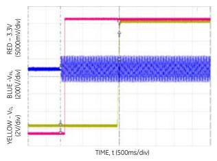
Figure 6. Typical Start-up ( $V_{IN} = 150V_{\alpha c}$ )
