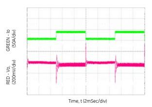
Figure 9. 10%-60%-10% Load Transient, Slew Rate = 1A/uS,  $V_{\rm IN}$  = 230Vac,  $V_o$  = 12Vdc
