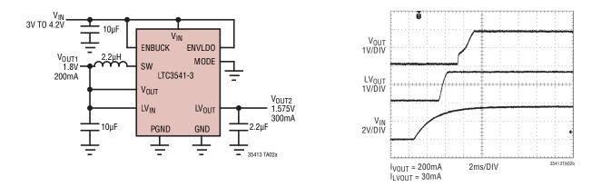
Dual Output with Minimal External Components Using Auto Start-Up Sequence, Buck in Pulse-Skip Mode for Low Noise Operation
