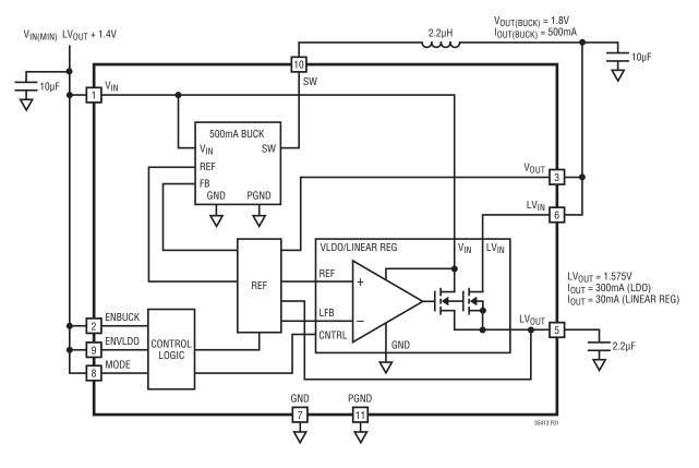
Figure 1. LTC3541-3 Functional Block Diagram
