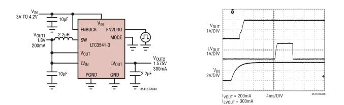
Dual Output Using Minimal External Components with V<sub>OUT2</sub> Controlled by External Logic Signal, Buck in Burst Mode Operation for High Efficiency Down to Low Load Currents
