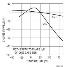
Figure 7. Change in Capacitor vs Temperature
