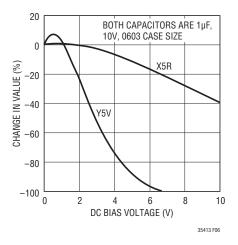
Figure 6. Change in Capacitor vs Bias Voltage
