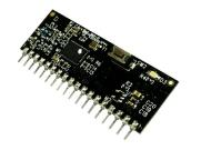
**BRAVO-T868** - 868 MHz SMART Radio Module with 8 digital outputs.
