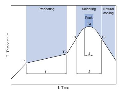
Preheating Soldering Peak Temp. Temp. Time Time Temp. Time T1 Т2 **T**4 t1 ТЗ t2 t3 150°C 180°C 120s 230°C 260°C 10s max. 30s
