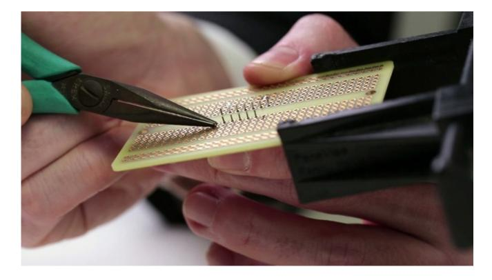
After placing a component on the board, bend its leads outward to keep it in place while soldering.
