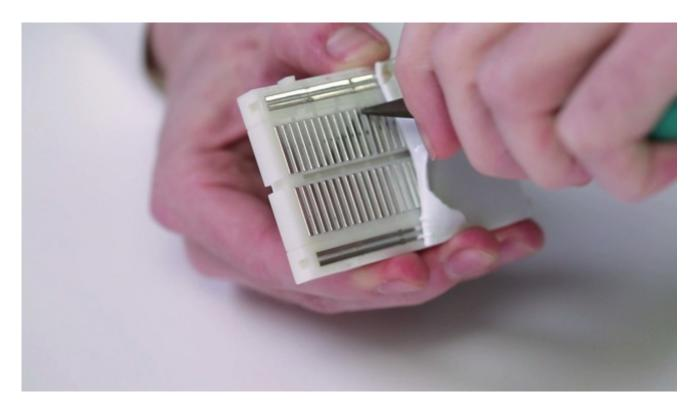
Beneath all those holes, a breadboard houses an army of springy metal clips which hold component leads in place while providing electrical connections between them.
