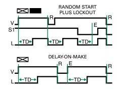
V = Voltage S1 = Initiate Switch L = Load (CR) E = Ready TD = Time Delay R = Reset
